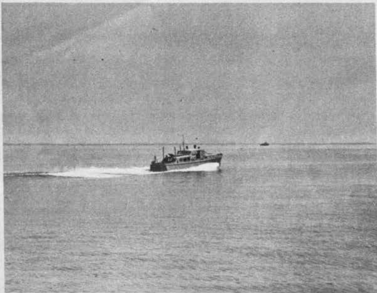
Shallow draft fits the 42-ft. picket boat for air-sea rescue in bays and harbors. Ample cabin, stepped down aft, makes it look like a peacetime pleasure craft. Cruising in friendly waters, it needs no armament.
